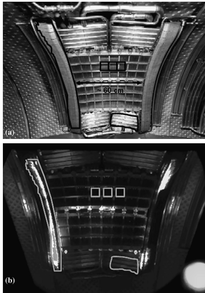
Fig. 4. Infrared monitoring of the lower hybrid couplers temperature during plasma discharge: (a) visible and (b) infrared imaging.
